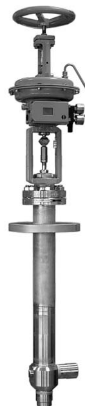
Fig. 2 Type 3248-7 Pneumatic Control Valve, angle valve with positioner, supply pressure regulator, pressure gauges and additional handwheel
